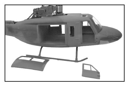
4.15 Mount the cockpit as shown using epoxy adhesive.
