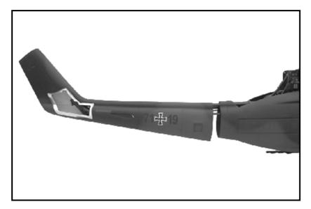
4.10 Install the tail propeller.
