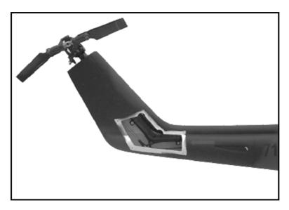
4.11 Screw the mechanism using the brackets (17) as shown.
