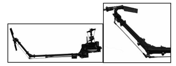
4.8 Then dismantle the tail rotor and linkage as shown for installation.
