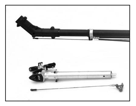
4.9 Insert the mechanics into the fuselage as shown.
