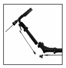
4.7 Install the tail servo and adjust the tail linkage and servo.
