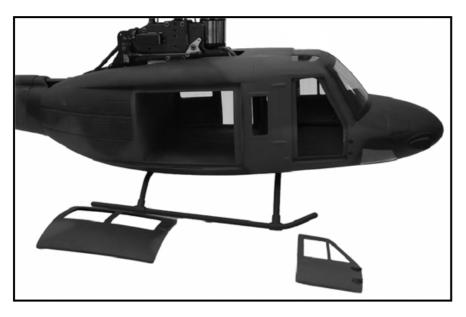
4.17 Pre-assemble the cockpit as shown.
