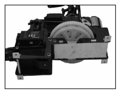
4.5 Install the tail struts as shown.
