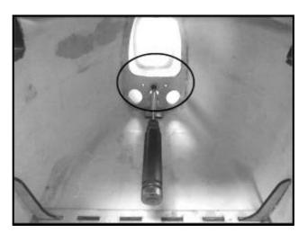
4.4. Attach the brackets with Screw A2x8 as shown.
