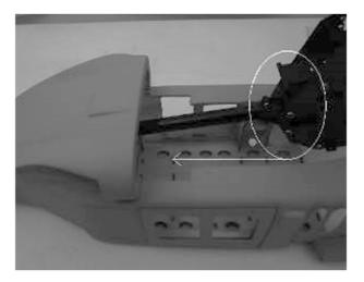
4.12. Install the tail propeller. Attach it with the wooden holder and 2 pieces of Screw A2x6 and the fuselage.
