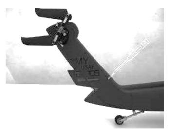
4.15. Install the mechanics with 2 pieces of Screw A2x8.
