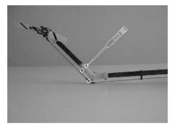
4.9. Install the mounting blocks as shown.
