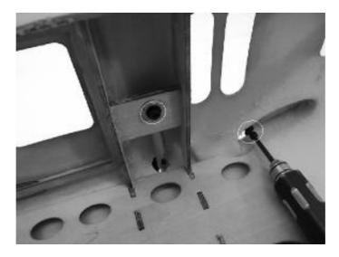
4.2. Assemble the landing gear as shown.
