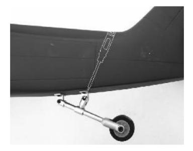
4.6. Secure the ball head with Screw M2x8 as shown.
