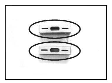
4.6 Mount the wooden holders on the mechanism as shown.
