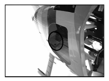
4.10 Secure the front section with 2 pieces of Screw A2x10 as shown.
