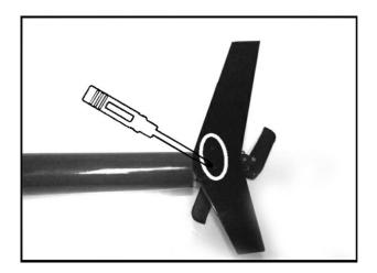
4.14 Glue the tail unit with epoxy resin adhesive as shown.
