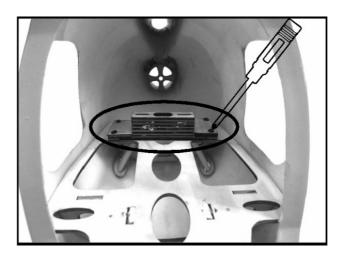
4.6 Remove the tail rotor from the mechanism.
