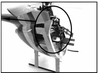
4.9 The wooden adapter must be inserted into the detent.
