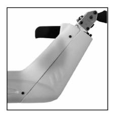
4.19. Glue tail wings into the fuselage with epoxy.
