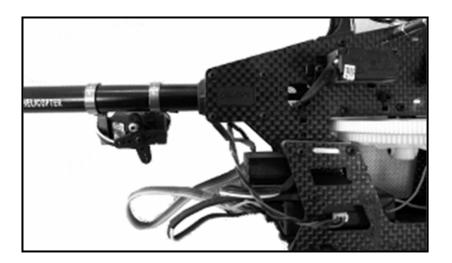
4.6. Remove the tail rotor frame.
