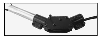
4.8. Assemble the tail boom as shown. Make sure belt isn't twisted twice.
