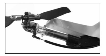
4.16. Adjust properly then drill 1mm holes through
