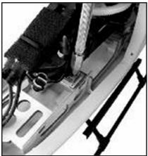
4.17. Tie down mechanics with screws.
