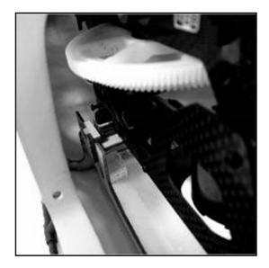
4.15. Flip tail upwards and tighten screw.
