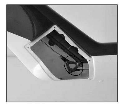
4.20 Adjust the position of the mechanism.
