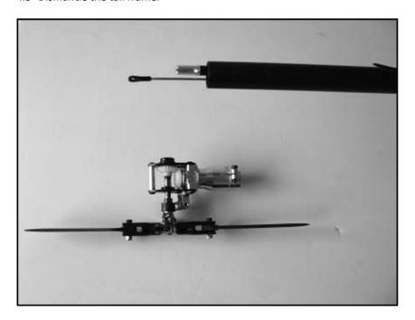
4.6 Mount the short tail tube and the linkage.
