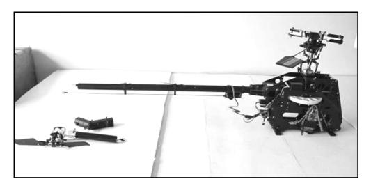
4.11 Mount the mechanism in the fuselage.
