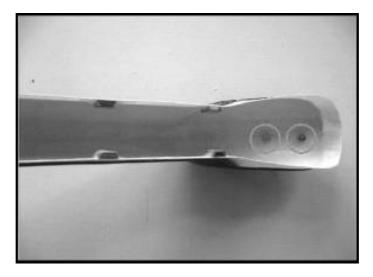
4.15 Screw the mechanism in the fuselage with 4 pieces of Screw M2x12.
