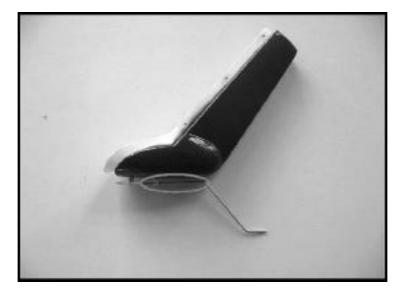
4.17 Secure the tail skid with Set Screw M3 as shown.
