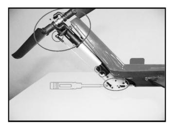
4.13 Install the tail distancer holders in the tail cover as shown.
