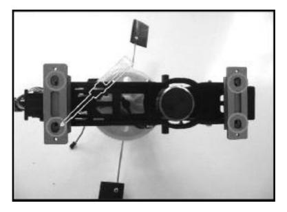
4.11 Install the mechanism in the fuselage.
