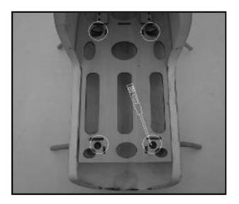
4.3 Install the T-connectors as shown.
