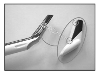
4.7 Install the tail control and test it first.
