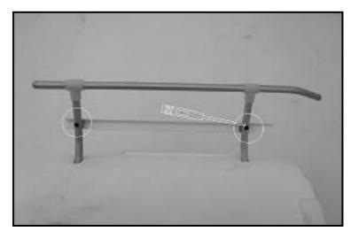
4.6 Remove the tail cover with Screw A2x12.
