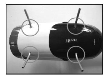
4.2 Secure the landing gear with 4 pieces of Screw M3x14 as shown.
