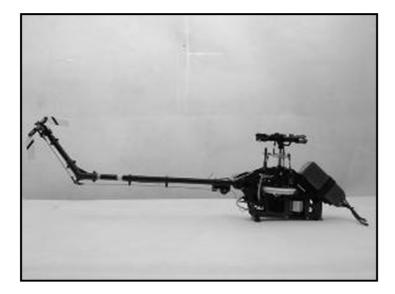
4.8 Loosen the screw as shown and pivot the tail.
