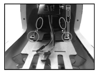
4.13 Install the linkage holders in the tail cover as shown.
