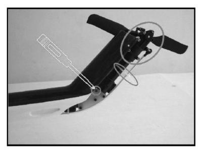
4.12 Install the mechanism in the fuselage with 4 pieces of Screw A2x12.
