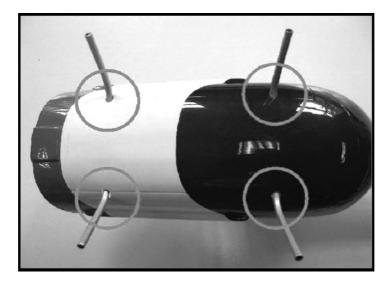
4.2 Secure the landing gear with 4 pieces of Screw A2x12 as shown.
