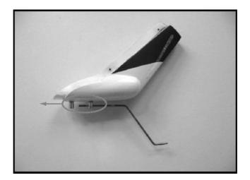
4.16 Secure the tail skid with Set Screw M3 as shown.
