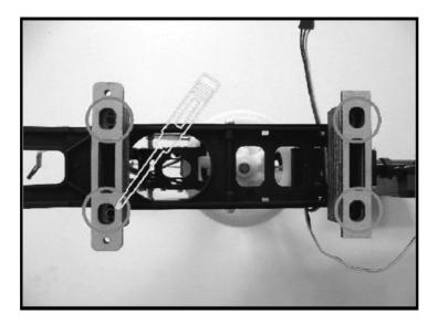
4.9 Secure the tail control with cable ties as shown.
