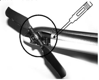
4.9 Mount tail fin as shown using screw A1.7x7.
