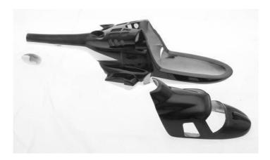
4.6 Take off the tail frame off the mechanics and insert it into the body as shown.
