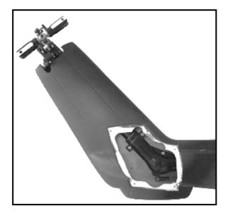
4.16. Install the linkage on the gearbox.
