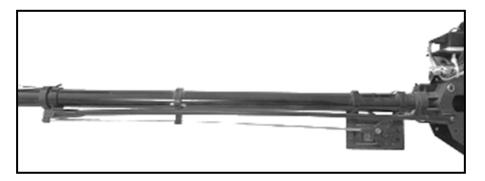
4.9. Install the rear gearbox as shown. Fly the mechanics with the 3D landing gear and check everything without the fuselage.
