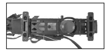
4.11. Remove the tail gearbox as shown.
