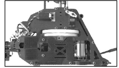
4.8. Mount the pushrod for the tail with the guide rings as shown.
